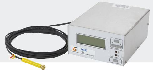
The Trek<sup>®</sup> 541A electrostatic voltmeter provides accurate non-contacting measurements of the electrostatic surface voltage associated with EOS/ESD processes. The instrument is configured with a miniature electrostatic field chopper probe that can be remotely located and easily positioned within process equipment to provide highly accurate, non-contacting, DC-stable, spacing-independent voltage measurements in either ionized or non-ionized environments.
