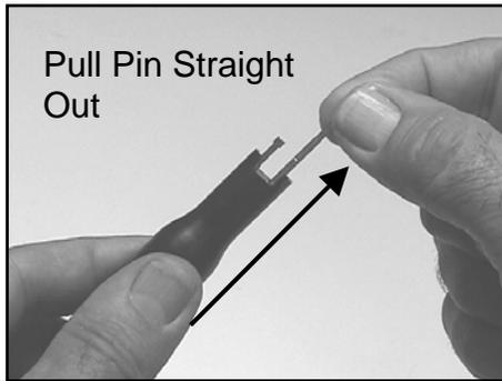
**Figure 11: Remove Spring-Loaded probe electrode by grasping firmly and pulling straight out of its socket.**
