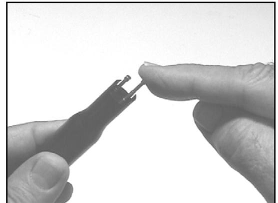
**Figure 13: Insert Test Probe into its Socket and Press Firmly to fully seat**
