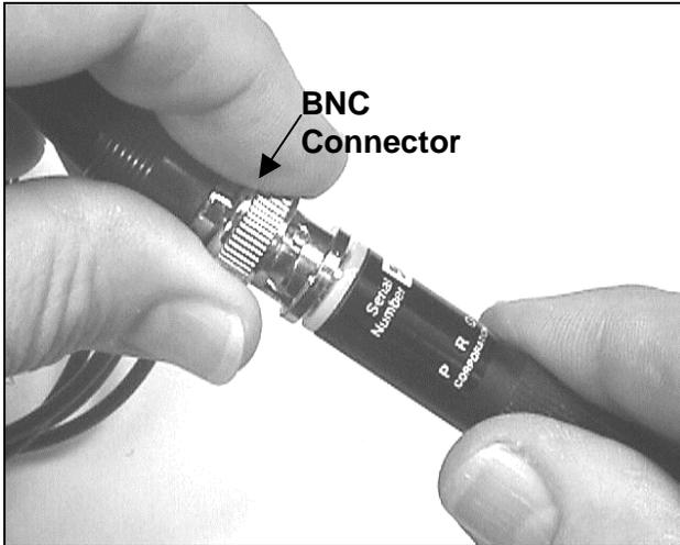
**Figure 2: Connect shielded cable to PRF-922B's BNC fixture**
