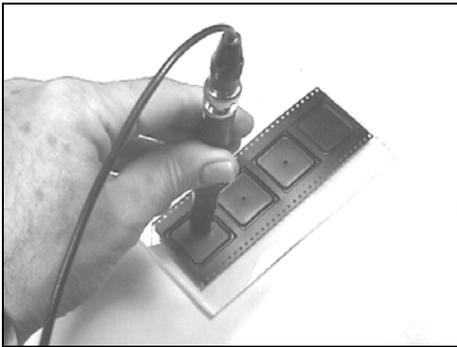
**Figure 7: Measuring Carrier Tape**
