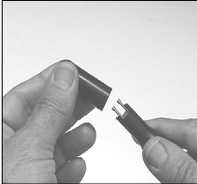
**Figure 5: Remove Probe Cover**
