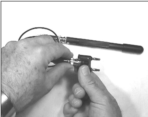
**Figure 3: Connect Cable to Banana Converter**
