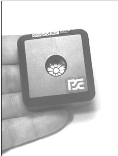
**Figure 4: PRV-913B Resistance Verification Reference**
