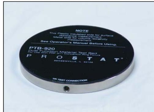
**Figure 3: Dual Test Bed**
