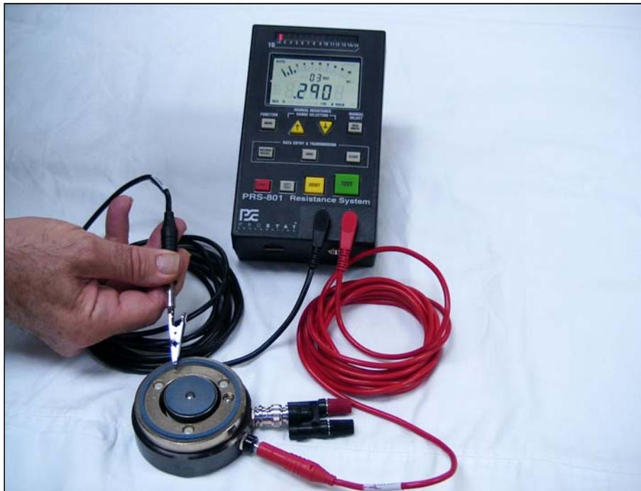
**Figure 7: Confirming Outer Electrode**
