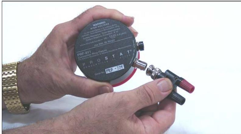
**Figure 2: BNC adapter and connection**
