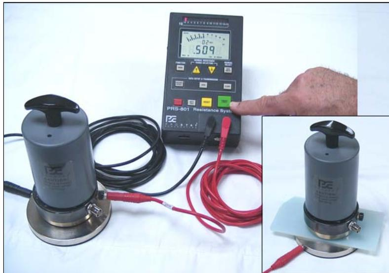
**Figure 9: Confirming Electrode Contact to Test Bed**
