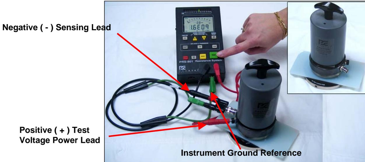
Figure 10: PRF-911 Fixture Preparation
