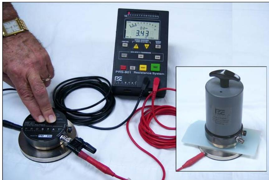
**Figure 8: Confirming Electrode Contact to Test Bed**
