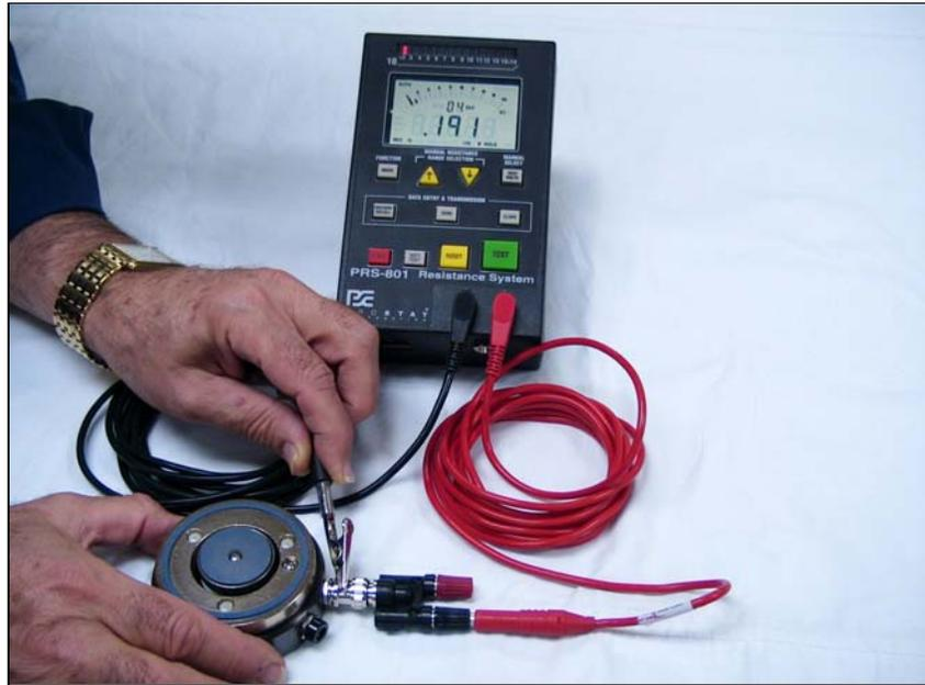
**Figure 5: Confirming Fixture Ground & BNC Connection**
