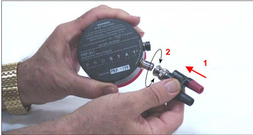
**Figure 4: Installing the BNC Adapter**
