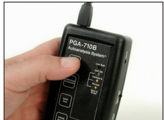
Figure 8: ON/OFF: Power up or place PGA-710B into "sleep mode".
